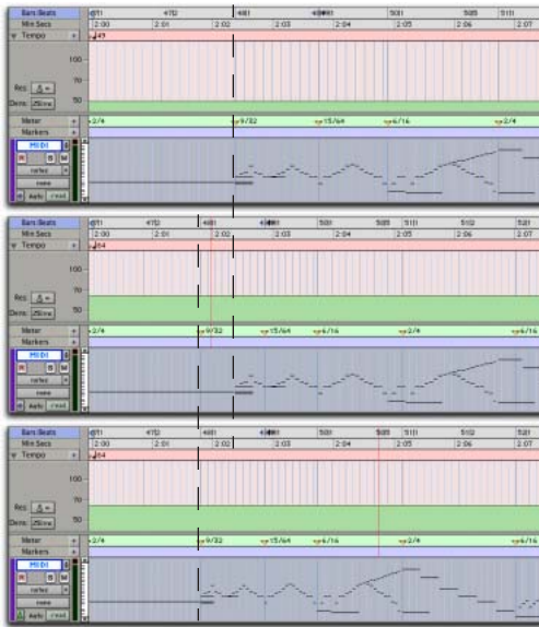
Figure 1. Top: Sample-based MIDI at 49 bpm, Middle: Sample-based MIDI at 64 bpm, Bottom: Tick-based MIDI at 64 bpm
