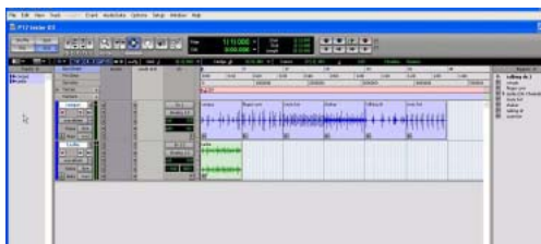
New tracks created by dropping multiple Region List items with Timeline Drop Order set to Left to Right mode
