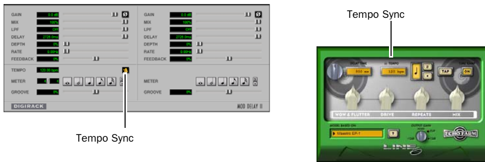
Figure 2. Tempo Sync control in Digidesign Mod Delay II (left) and Line6 Echo Farm (right)
