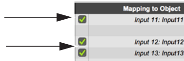
Mono bus mapped to Object 11, and Mono sub-paths of stereo bus mapped to Objects 12 and 13
