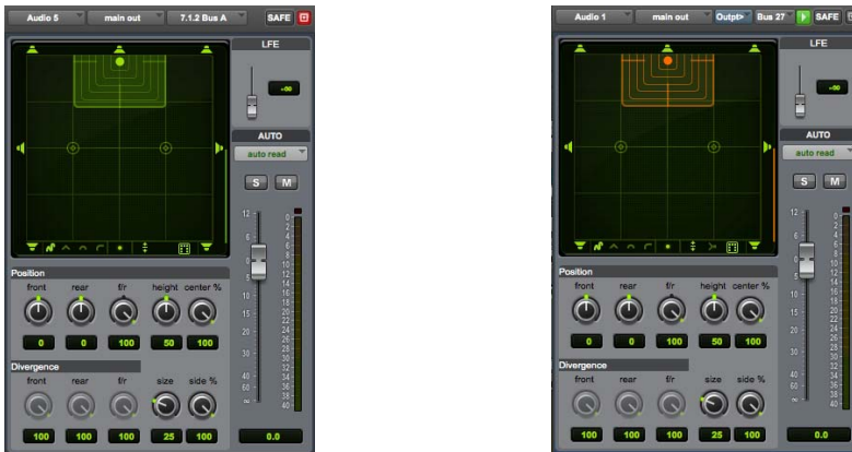
Figure 2. Output window in standard (2D) view for a mono track assigned to a 7.1.2 bus (left) and an Object (right)
