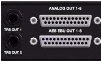
Back panel analog TRS outputs, and analog and digital (AES/EBU) DB-25 outputs
