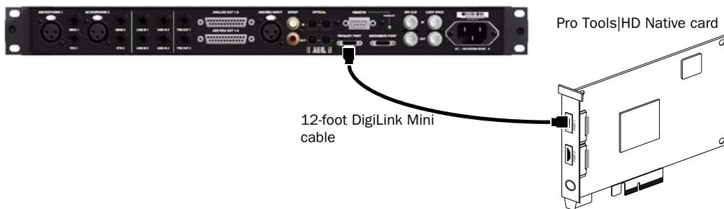
Figure 3. HD OMNI connected to the DigiLink Mini Port 1 on a Pro Tools|HD Native card (8-channel system)
