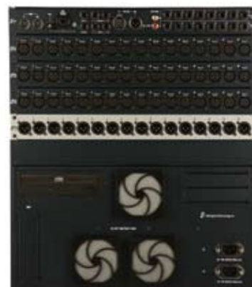
Mix Rack back panel
